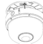
7. Twist the camera counterclockwise until it is secured firmly in place. Then fix the camera on the ceiling with the screw.
