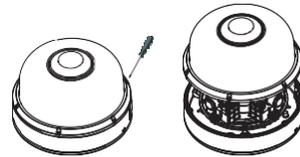
2. Remove and discard the protective EPE from the lens modules.
