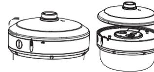
7. Loosen the 3 anti-drop screws on the bottom plate and open it.
