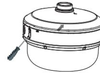
6. Rotate the cap (▽) from LOCK to OPEN in order to remove the cap.
